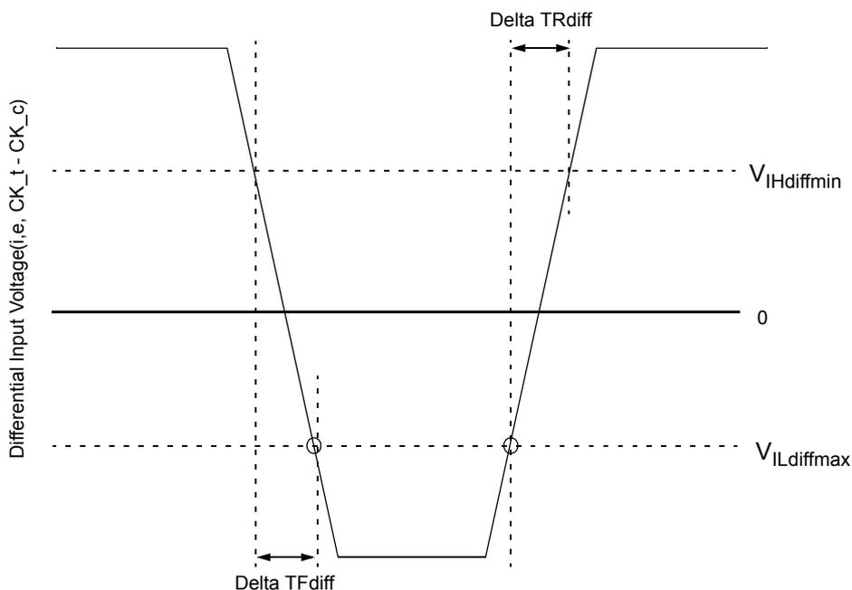
Figure 7. Differential Input Slew Rate Definition for CK<sub>t</sub>, CK<sub>c</sub>
