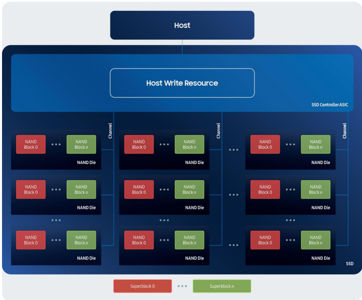
Figure 1. Typical Conventional NVMe SSD
